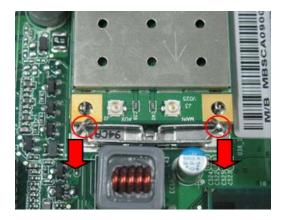
**b.** take off wireless LAN card from M/B MINI-PCIE" connector.
